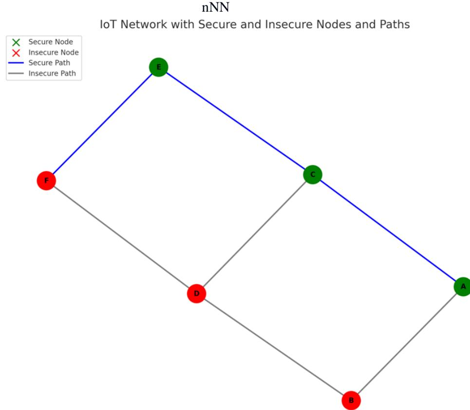
**Note:** The nodes are marked as secure (green) or insecure (red), while the edges in blue represent paths protected by secure routing protocols.
